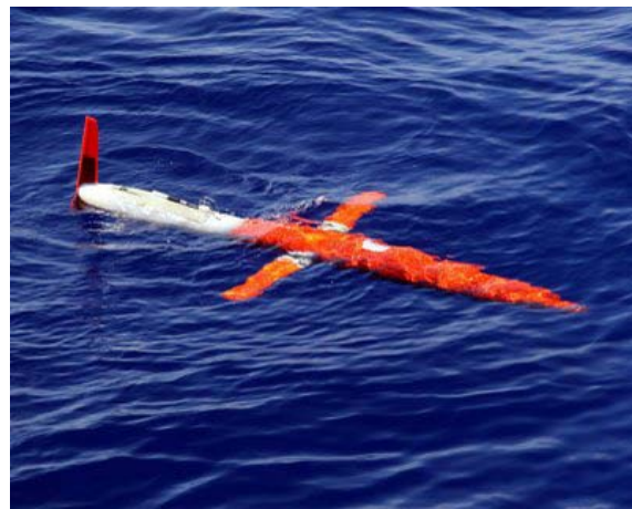
The underwater glider, "Spray": 7' long, 8" diameter.
