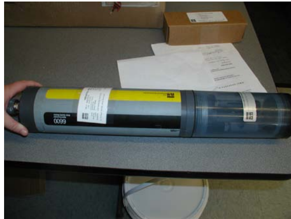
The YSI 6600 to be deployed.
