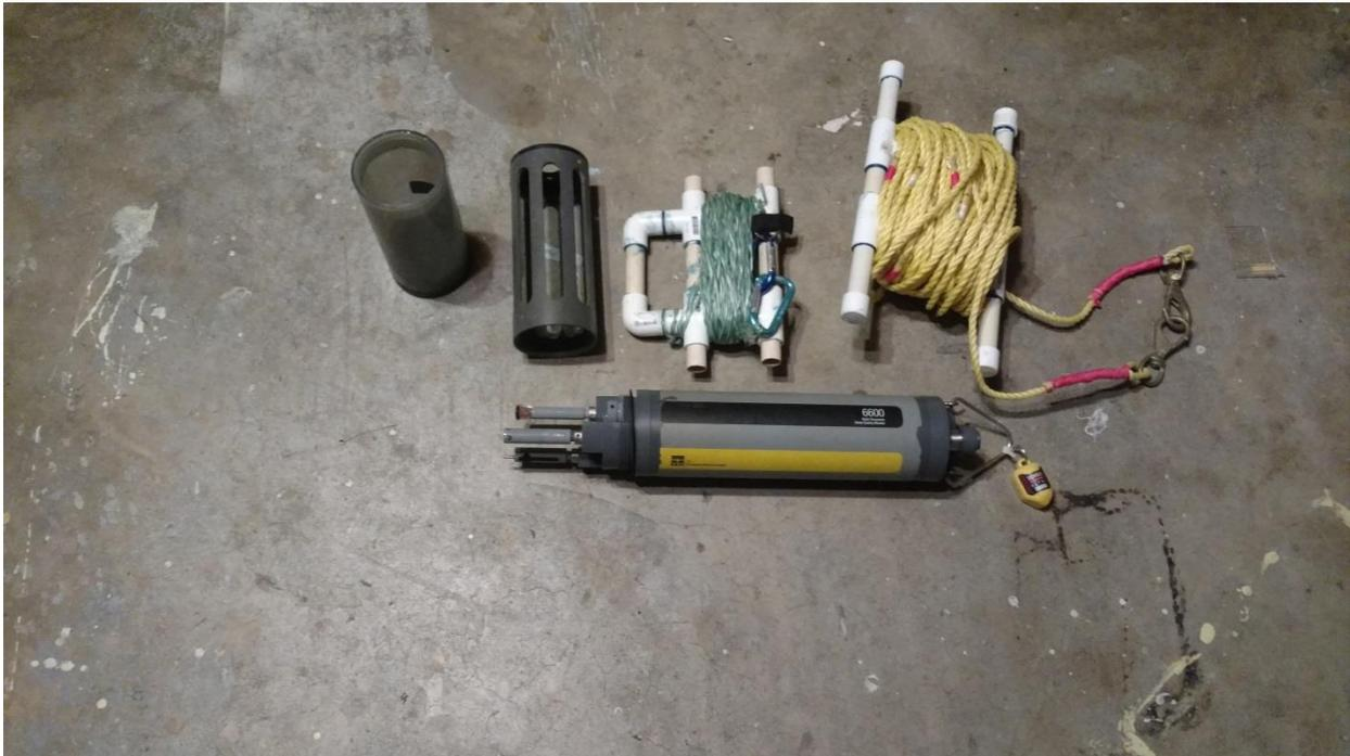
5. Place the calibration cup in the gear bag and take the cage out. The cage must be screwed onto the sonde, replacing the calibration cup. The cage permits sea water to reach the sensors.
